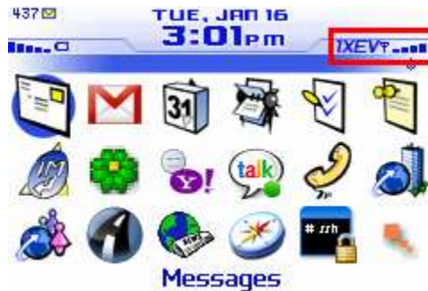
This BlackBerry is receiving a data signal on the EVDO network with four bars of strength.
